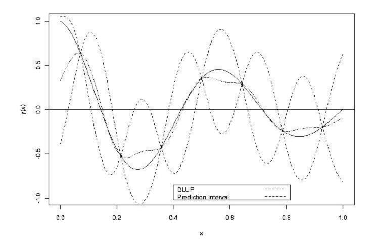
The BLUP and corresponding pointwise 95% prediction interval limits for y(x) for n = 7 training data observations
