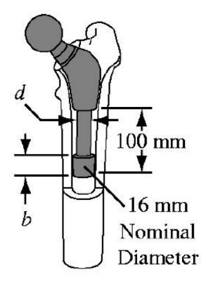
**Goal** To determine the design of a hip implant, i.e, (b, d) that minimizes femoral stress shielding while providing adequate resistance to implant toggling.
