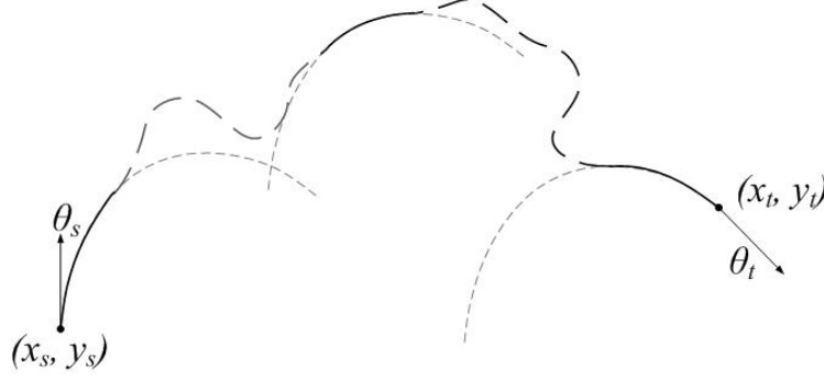
Figure 3.16: An optimal path consists of the segments making up the curve \mathcal{C}_R(\theta_s, \theta_t) (bold solid lines), and the remaining segments (bold dashed lines).
