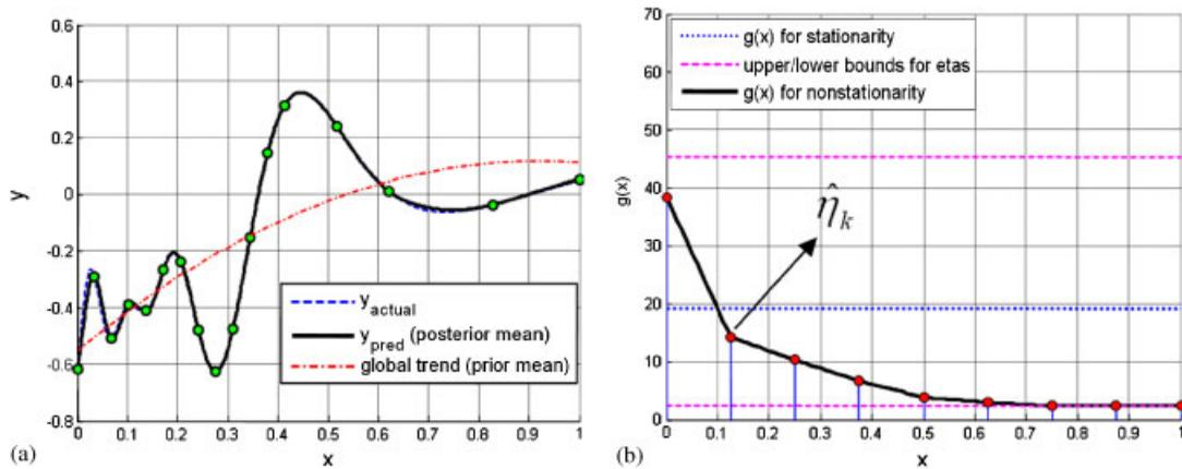
Figure 6. Results of non-stationary Kriging with piecewise linear density function ( $K = 8$ ): (a) Kriging prediction; and (b) estimated density function.
