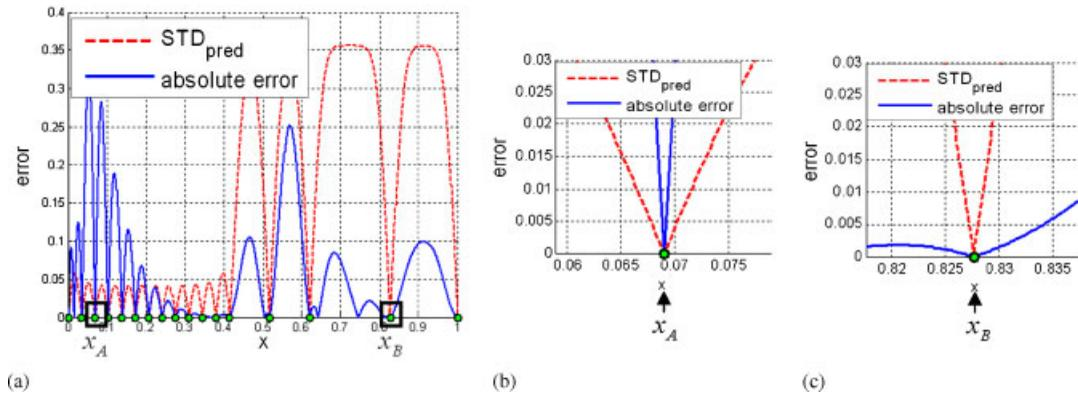
Figure 13. The theoretical standard deviation of prediction error vs the actual absolute prediction error yielded by stationary Kriging.
