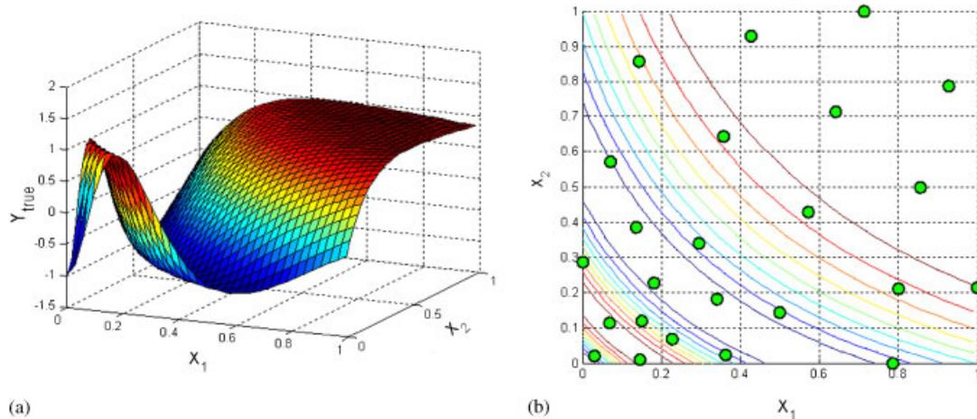
Figure 9. The true surface and adaptive sampling points (Function 3): (a) true surface; and (b) adaptive sampling points.
