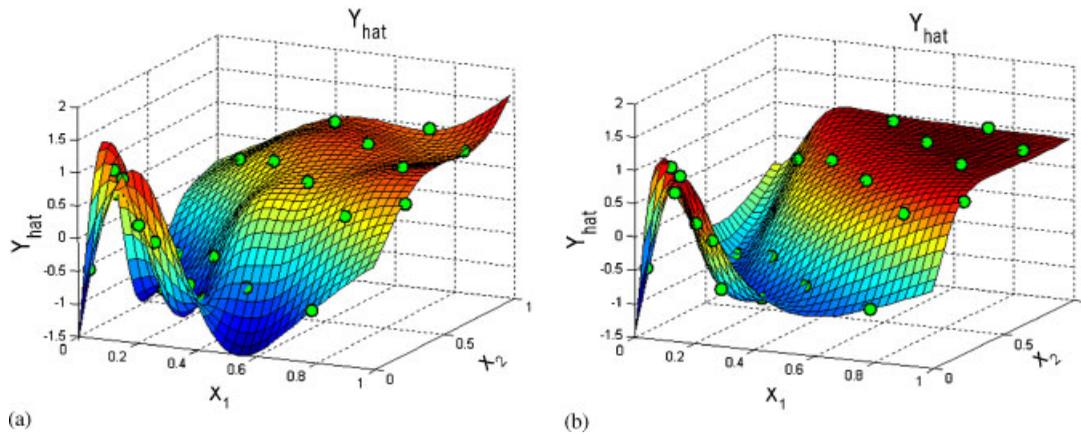
Figure 10. The predicted surface *via* the two Kriging models (Function 3): (a) stationary Kriging; and (b) non-stationary Kriging.
