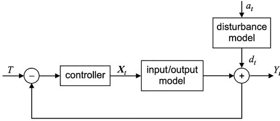
Fig. 1. Block diagram of assumed process model.
