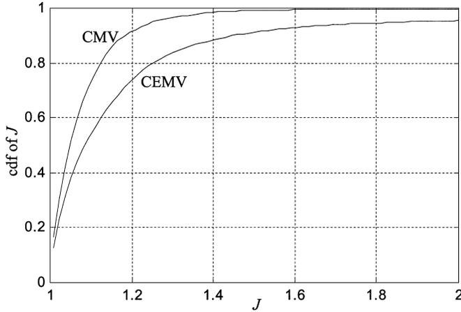
Fig. 5. Cdfs of the mean-square error  $J$  for CMV and CEMV control.
