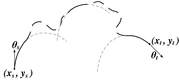
Figure 13: Conceptual example of an optimal path consisting of the segments making up the curve \mathcal{C}_R(\theta_s, \theta_t) (solid bold lines) and the remaining segments making up the sub-path (dashed bold lines).
