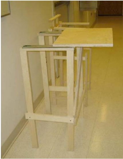
Figure 1. The walker tray design demonstrating the tray in the slid out position.
