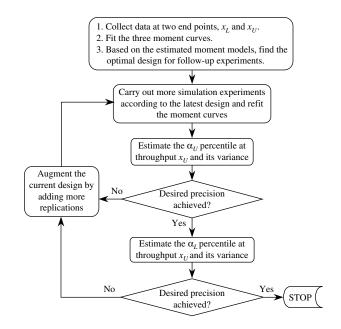
Figure 2 Flow Chart for the Multistage Procedure
